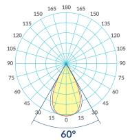
Peak emission wavelength: 222 nm Output power in range (200-230 nm): 115 mW Dose needed (222 nm, COVID-19) 90% inactivation for aerosols: 390 μJ/cm2 Dose needed (222 nm, COVID-19) 90% inactivation for surfaces: 600 μJ/cm2
