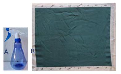
*Figure 3. Spray bottle for distributing bacteria evenly on surfaces (A). Distribution of sampling areas on gown fabric (B).*
