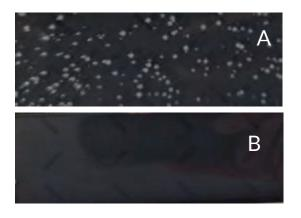
*Figure 6. Gown sample before irradiation (A), Gown sample after a dose of 10 mJ/cm.<sup>2</sup> (B).*
