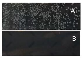
*Figure 7. Mask sample before irradiation (A). Mask sample after a dose of 10 mJ/cm<sup>2</sup> (B).*
