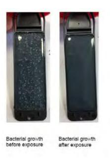
Figure 2. Bacterial count testing with Hygicult stripes.
