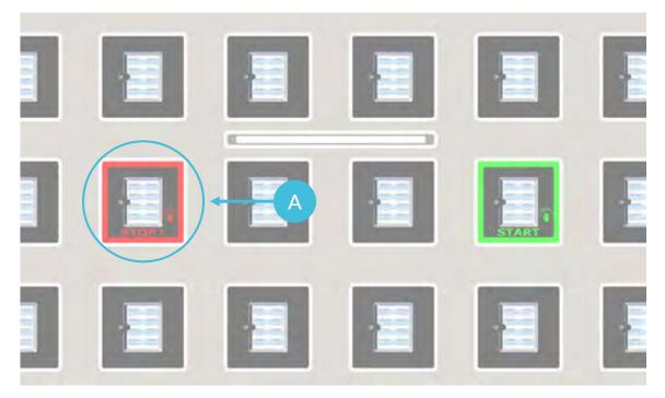
b) Cleaning stop: a grey stop button on the left side of the booth can be pushed when cleaning is needed.
