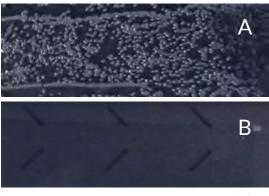
*Figure 8. Goggles sample before irradiation (A). Goggles sample after a dose of 10 mJ/cm<sup>2</sup> (B).*
