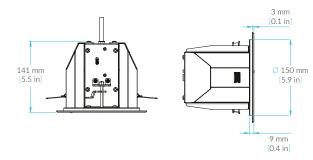
Once the Product is connected to a power source, push the side springs and insert in the opening made on the ceiling panel.
