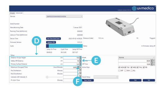
10) Save setup into template by pressing "Save Setup". A
